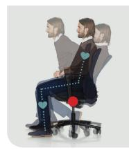
The HÅG centre-tilt mechanism (HÅG in Balance® have a centrally placed tilting- point which ensures that you always sit in balance, above the natural pivot point of the chair. The mechanism allows you to tilt backwards and forwards with equal ease, using your legs to control the movement.
